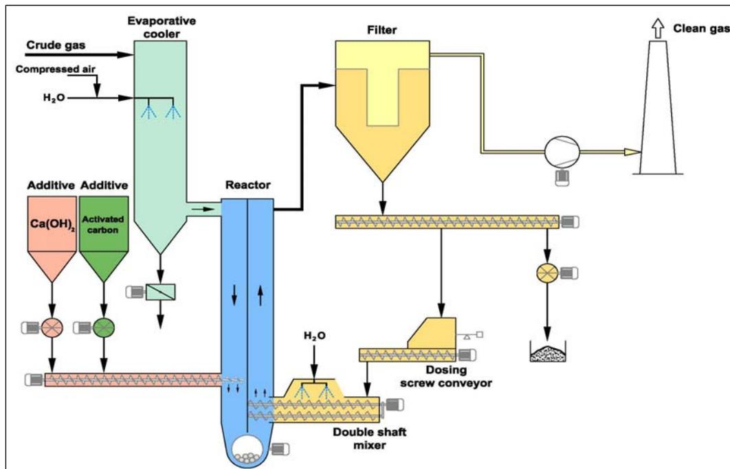
III. 3: Chemisorption with gas and particle conditioning
