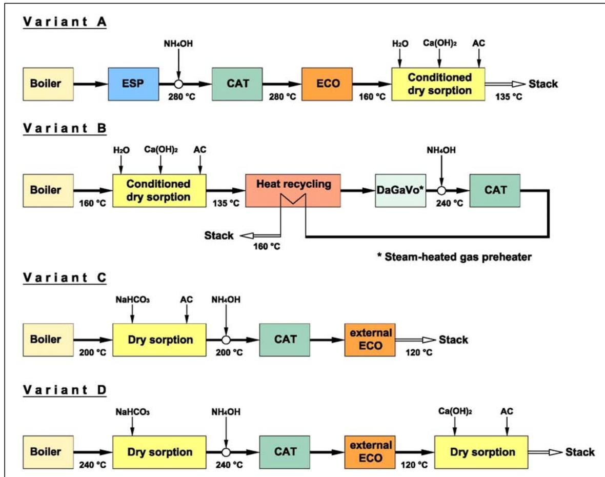
III. 1: Flue gas cleaning concepts with catalyst for  $\text{NO}_x$  reduction
