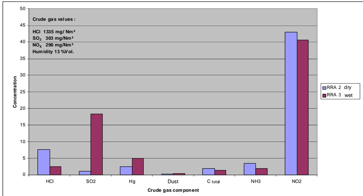
III 6: Comparison of gas cleaning systems „wet“ and conditioned dry“ (2005)
