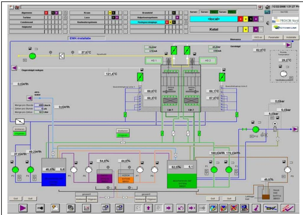
III 13: Wet ESP with integrated two-stage scrubbing
