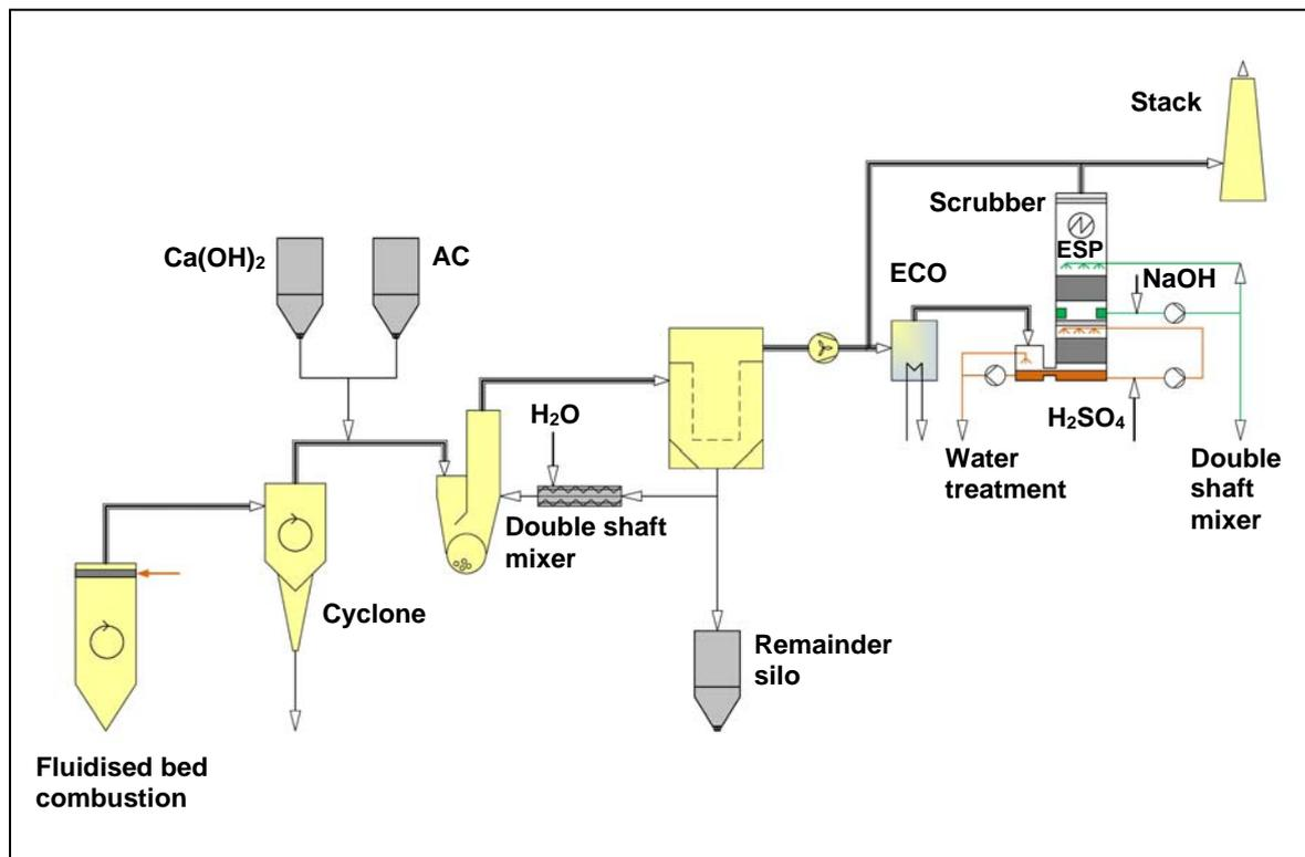
Ill. 11: Process concept for gas cleaning system at HVC Alkmaar
