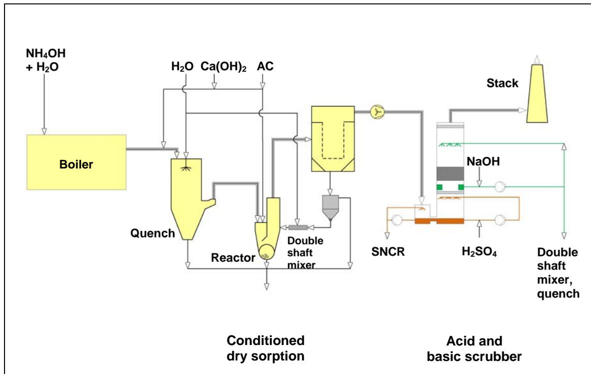
Ill. 8: TwinSorp process: Variant II: Combination conditioned dry sorption – acid and basic scrubbing
